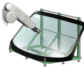
Curvature measurement of glass surfaces
