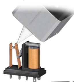
Operation inspection of relay contacts
