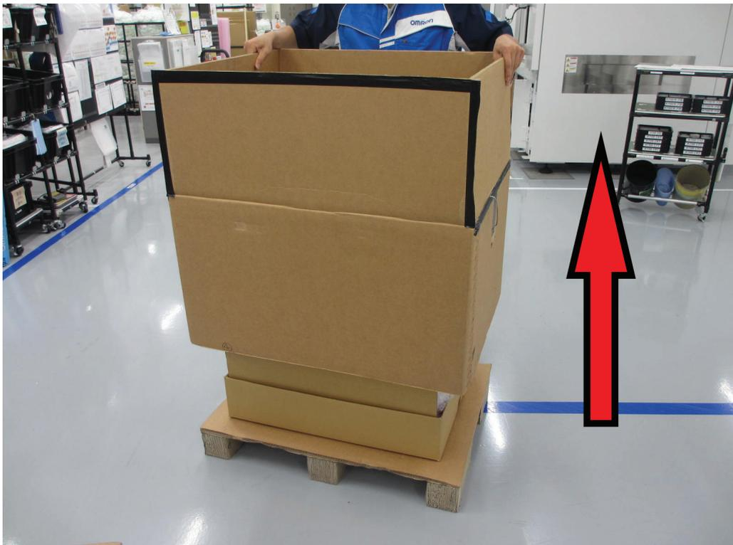
**7** Lift the robot using two people holding the grips at each side of the cardboard carrier.
