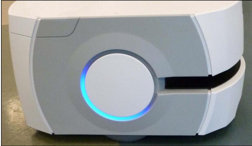
Figure 10-10. Right Side Cover, Showing Even Gaps at Edges
