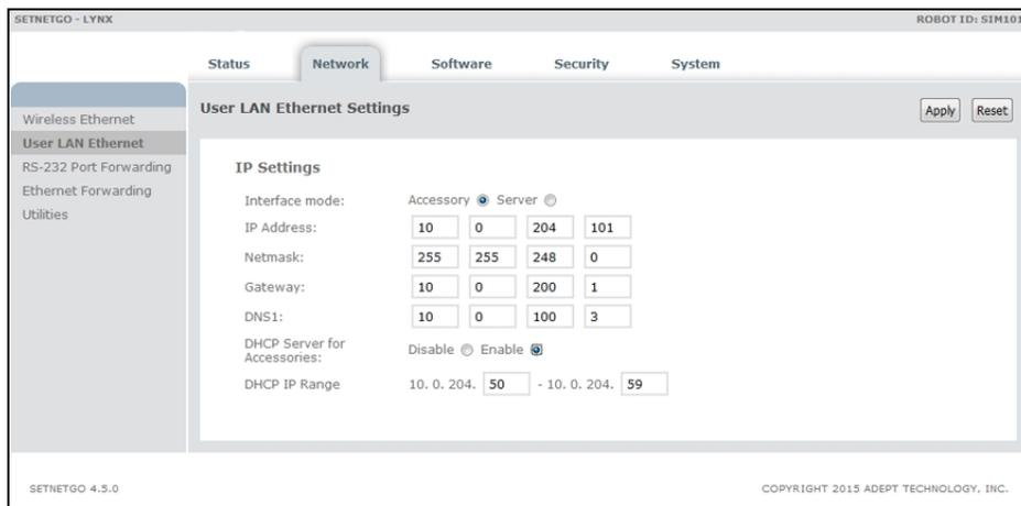
Figure 4-1. Accessory and DHCP Server for Accessories Enabled
