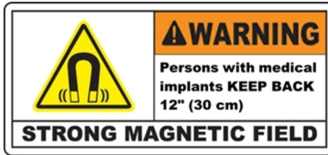
One magnetic field/implant label is on the transporter rear cover.
