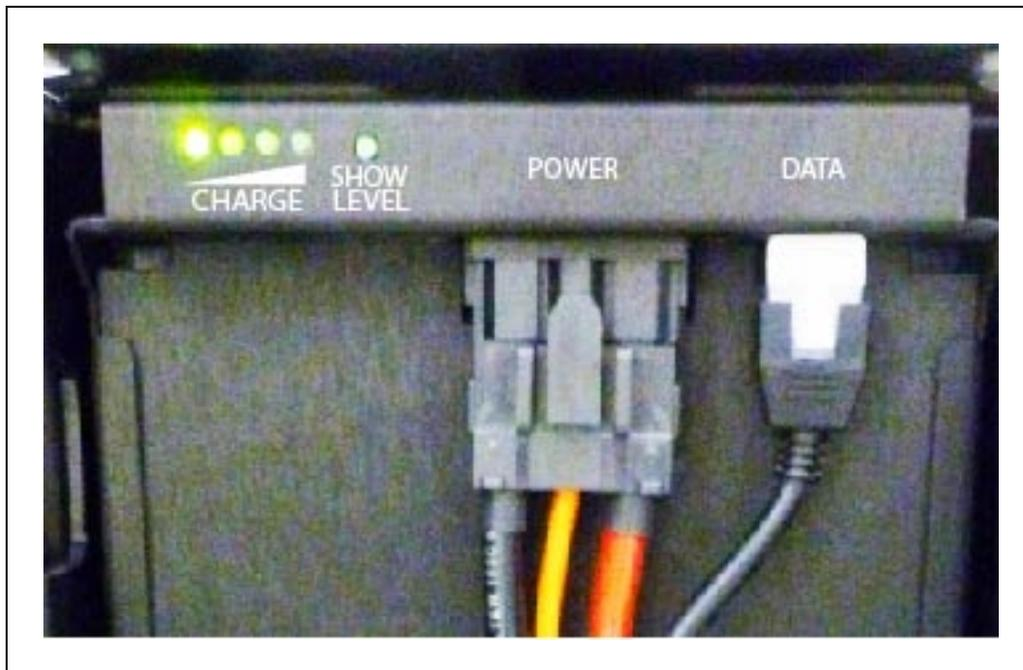
*Figure 3-14. Battery Cable Connectors*
