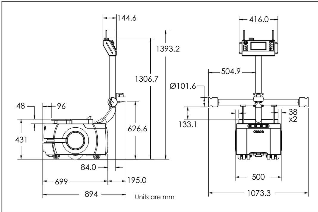
Figure 11-1. Overall LD Platform Cart Transporter Dimensions
