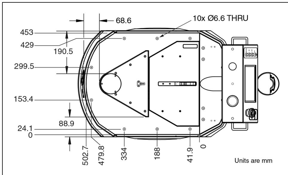
Figure 11-2. Coupling Plate Dimensions, Arms Removed
