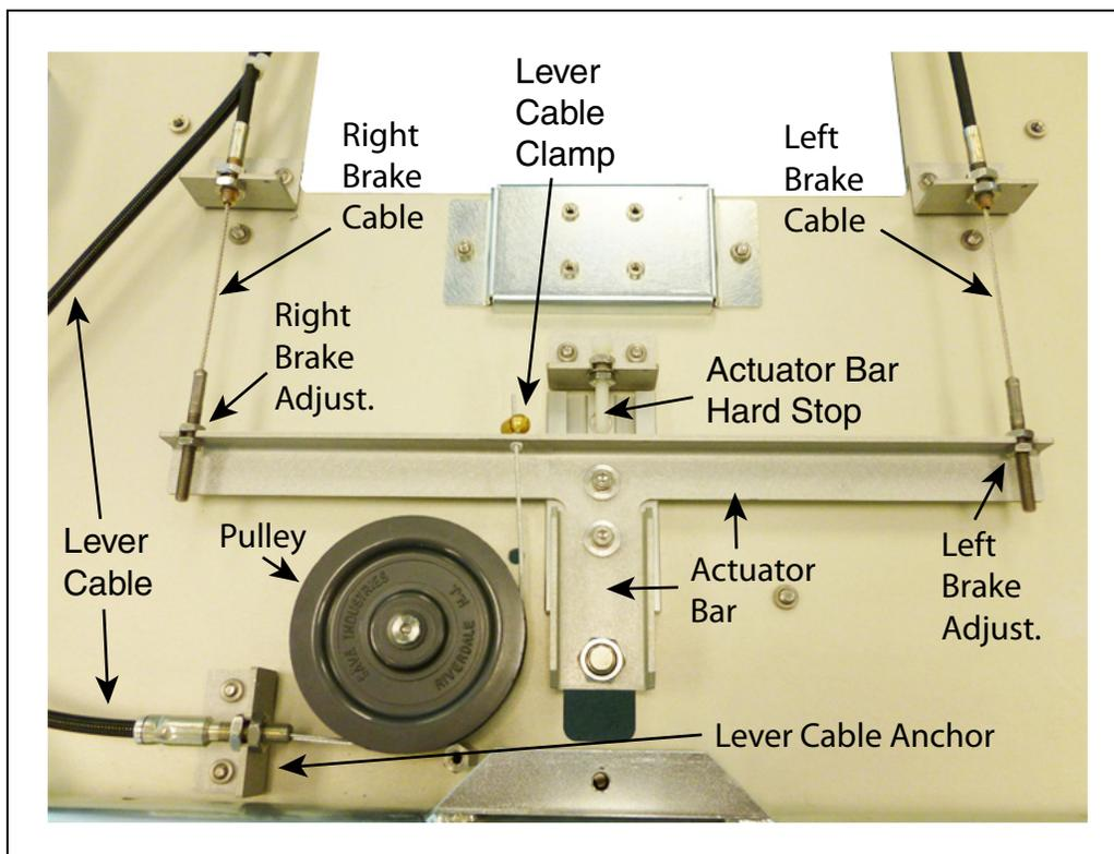
Figure 10-22. Internal Brake-Release Mechanism
