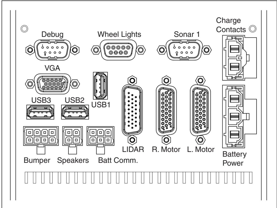
Figure 6-12. Internal Connectors on the LD Platform Core (Front)
