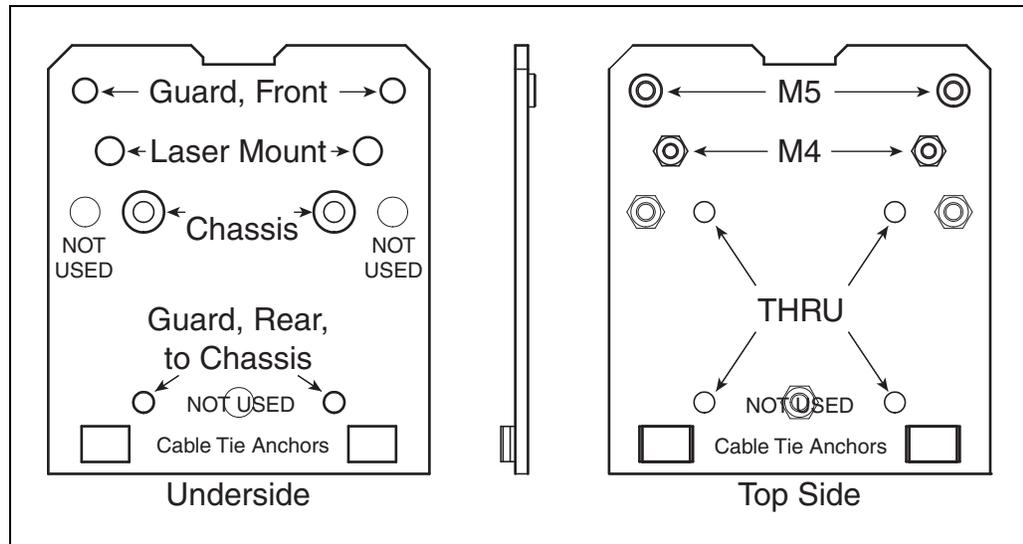
Figure 10-13. Mounting Plate for Low Front Laser and Guard
