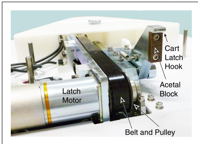
Figure 10-14. Cart Latch Mechanism with acetal block, Vertical Position
