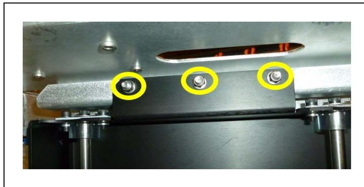
Figure 10-17. Mounting Studs and Nuts at top of Drive Assembly
