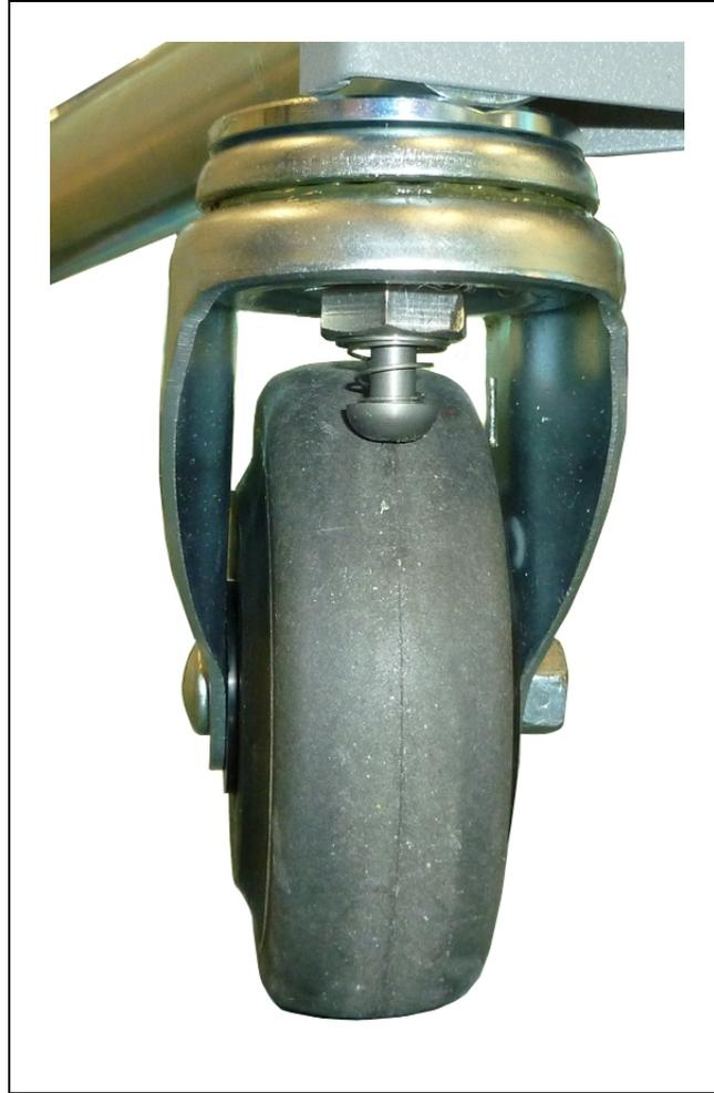
*Figure 3-21. Cart Caster Brake, Showing Spring and Pin*
