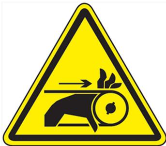
A hand entanglement label is under the latch mechanism cover, near the belt and pulley. See *Removing Latching Mechanism Cover* on page 151 for instructions on removing the cover.
