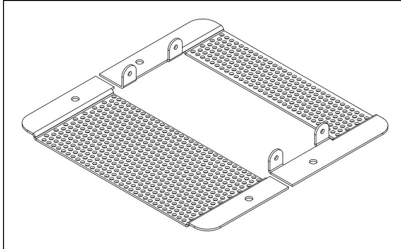
Figure 10-23. Core Mounting Bracket
