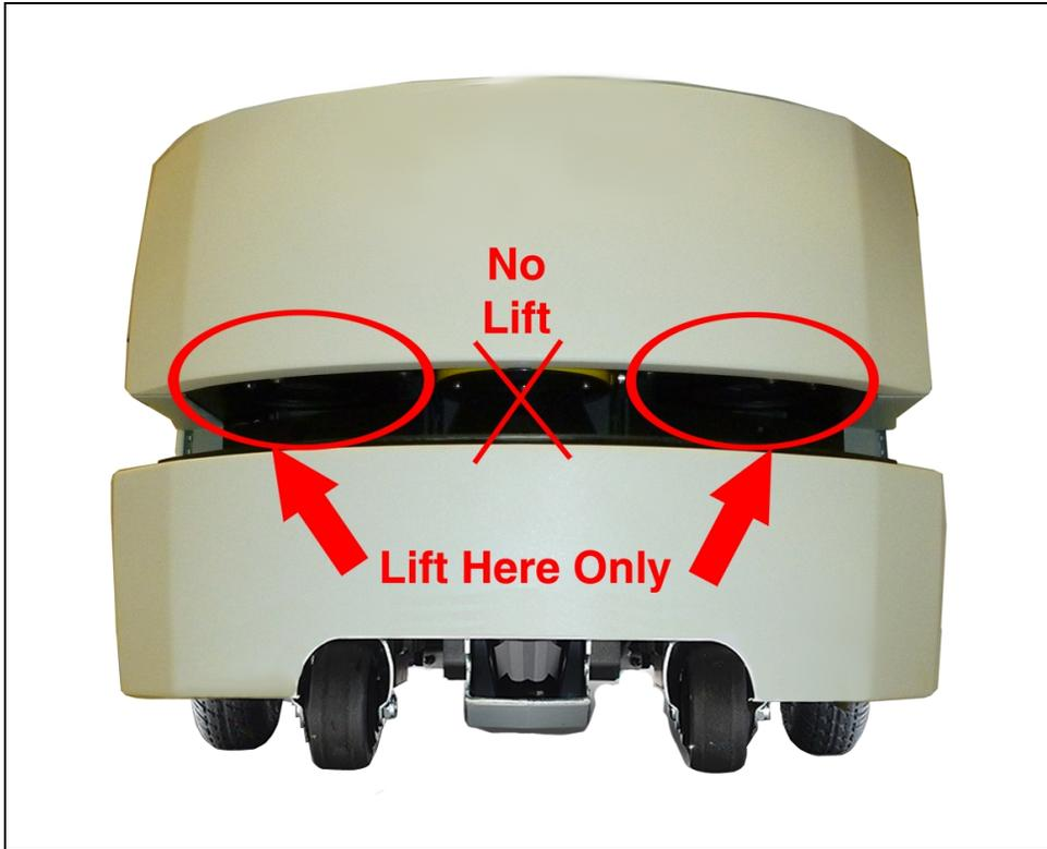
Figure 10-4. The upper surface of the laser slot, at both sides, not the center.
