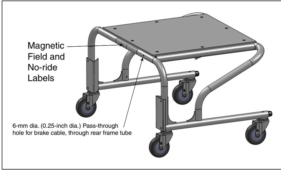
Figure 10-7. Magnetic Field/Implant, and No Riding Labels on Cart
