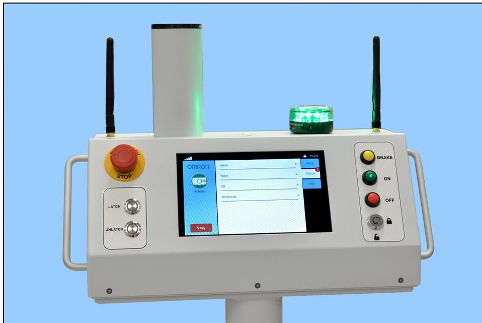
Figure 7-1. Operator Panel, with Acuity Option Shown
