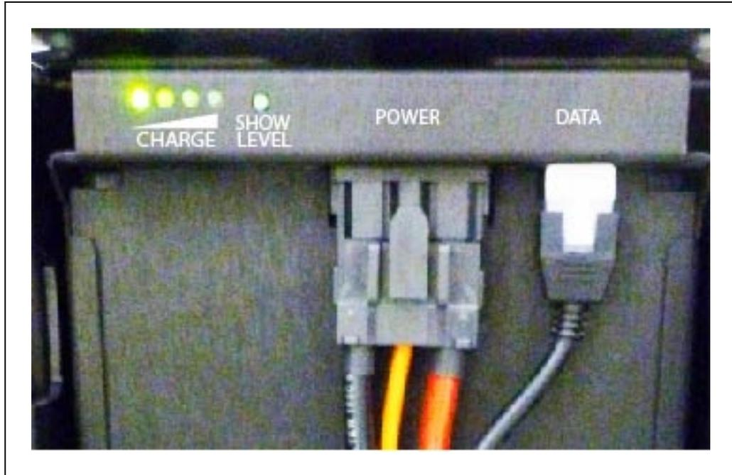
Figure 8-2. Battery LEDs, Push-Button, Power Cable, and Data Cable
