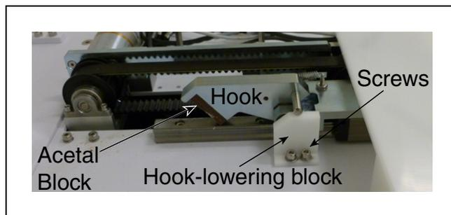
Figure 10-15. Hook-lowering Block and Screws
