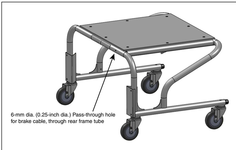
Figure 3-23. Thru-hole for Brake-release Cable
