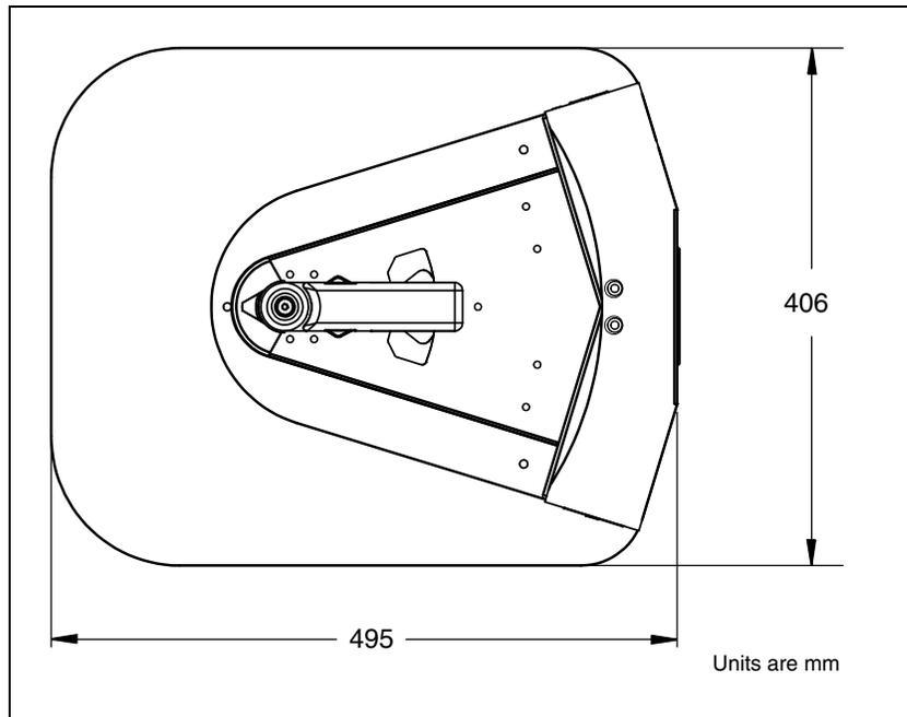
Figure 3-19. Docking Station Floor Plate Dimensions
