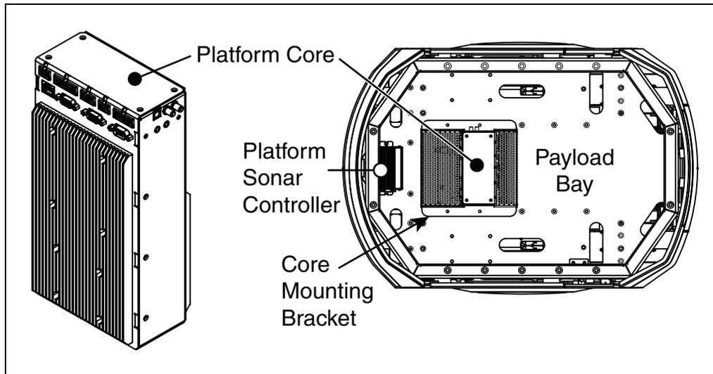
Figure 10-3. Location of Parts in the Payload Bay
