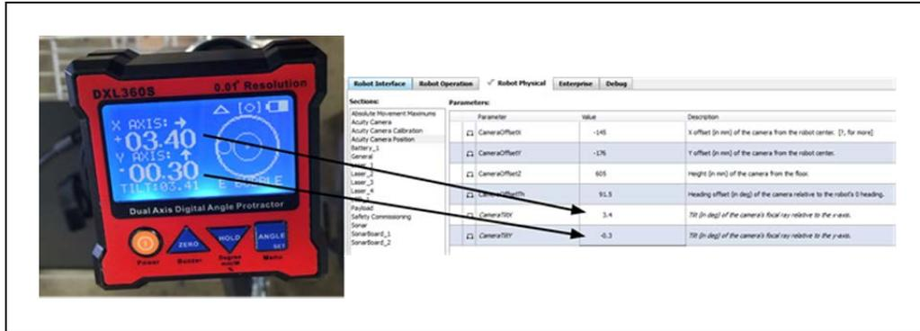
Figure 6-18 Transferring Level Readings to the MobilePlanner Software
