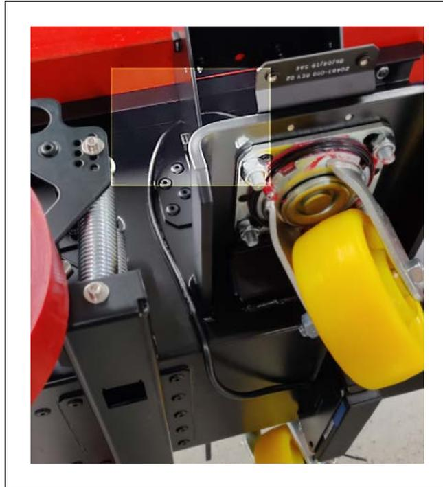
*Figure 9-15 LD-250 Front HAPS Cable Routing Behind the Speaker Mount*
