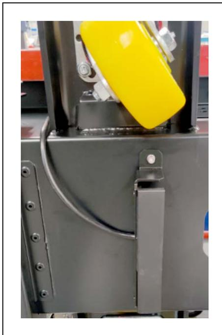
*Figure 9-14 LD-250 Front HAPS Cable Routing Over the Sensor Bracket*
