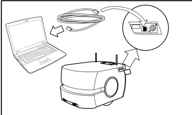
Figure 3-2: Ethernet Connection
