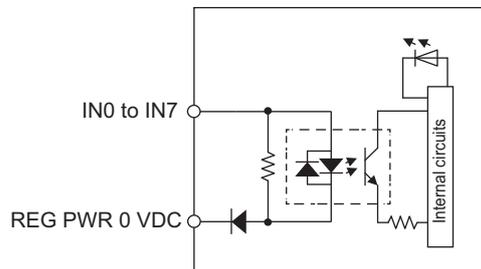
A circuit diagram is provided below for the analog inputs.
