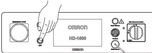
An LED ring around the button flashes red during the shut-down procedure.
