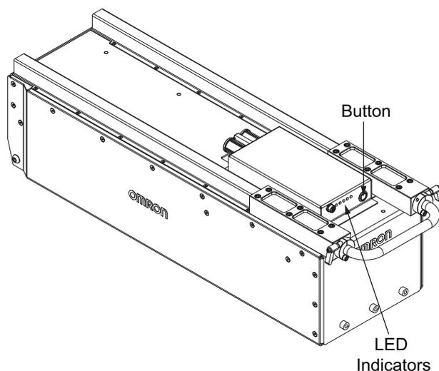
Pushing the button has different functions based on the battery location and the state of the AMR. When the battery is not installed in the AMR, press and hold the button until the LED indicators illuminate purple to display the state of charge (refer to the table below). LEDs will flash yellow while pressing the button to indicate a battery charge level request is in progress. Displaying the battery's state of charge with this method can be useful when a battery is in storage.
