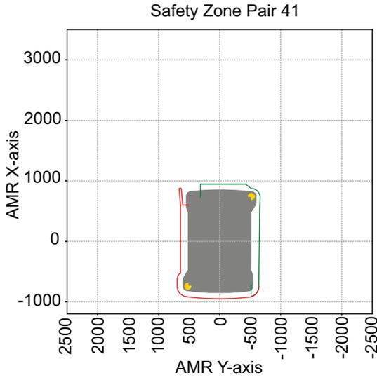
The following figure provides dimensions of the AMR unprotected area at the front of the AMR.
