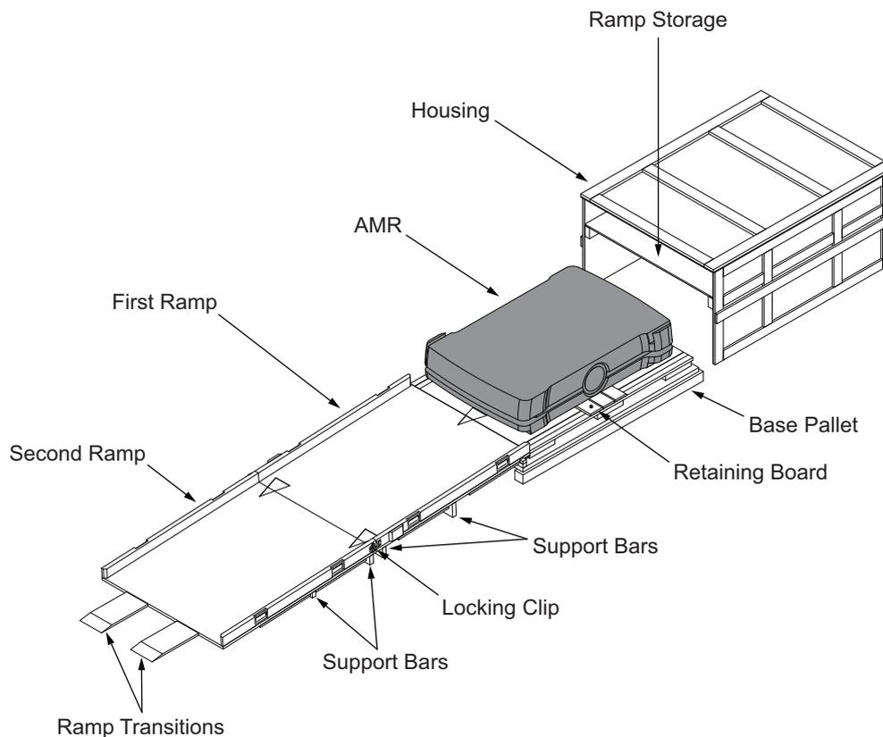
Before beginning this procedure, there must be at least 7 m of open area in front of the AMR shipping crate for unloading purposes. There must be 2 m of open area behind the AMR shipping crate to allow the housing to be pushed back.
