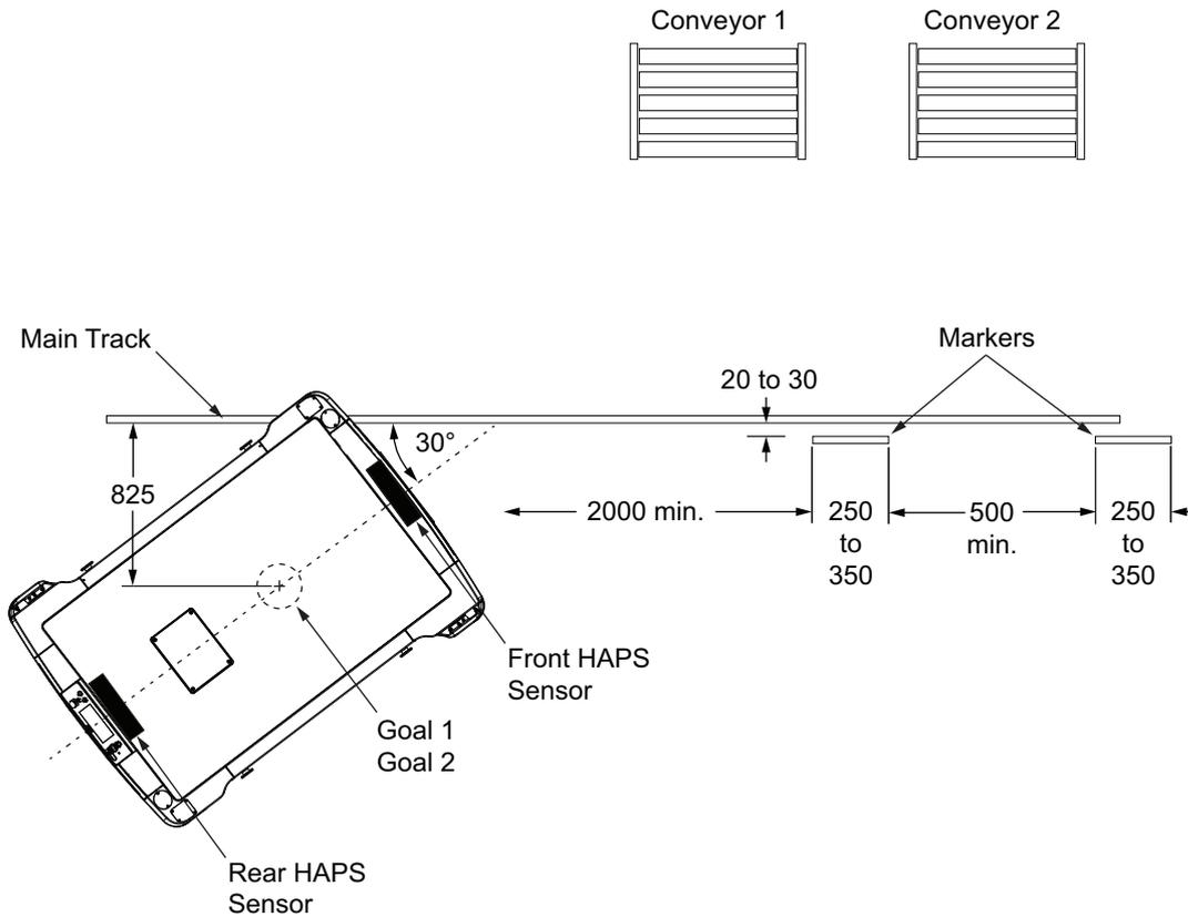
If you use the same magnetic tape for markers as for the main tape strip, apply the markers upside-down, relative to the tape. If you use tape with North side up ensure that the markers are applied with their South side up.
