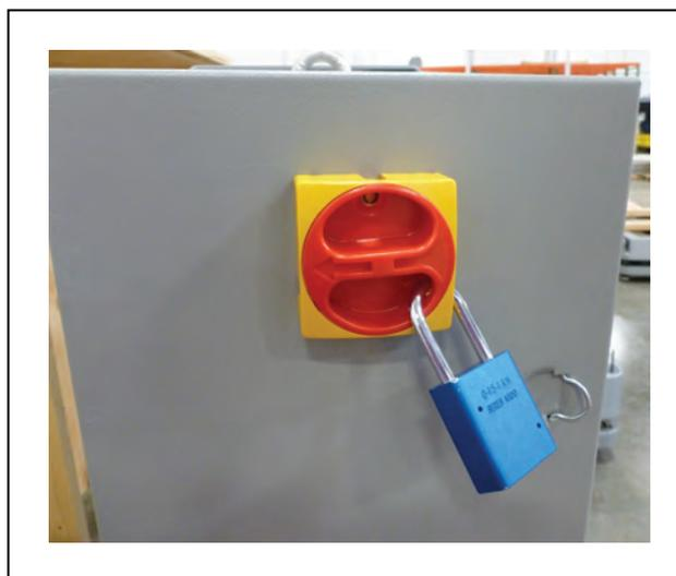
*Figure 2-16. Main Disconnect Switch Locked*
