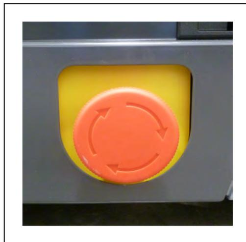
*Figure 2-4. E-Stop Button on the Platform*
