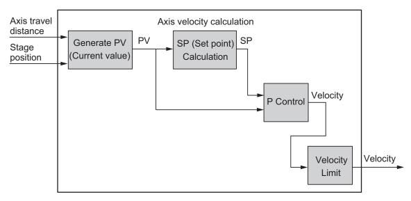
PV and SP are values generated to calculate the velocity inside the FB and are never output outside the FB.
