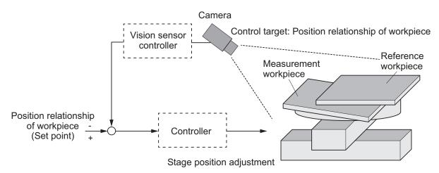
This library is a set of software components (Function Blocks (FB) / Functions (FUN)) that realizes the alignment application with visual feedback. By combining FB / FUN provided with this library, it is possible to build alignment control that applies visual feedback with the user program on the controller.
