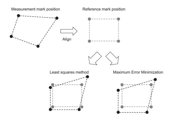
The values output to the X and Y coordinates of the reference mark position (for alignment control) and the measurement mark position (for alignment control) become the center of gravity of the input reference mark position (stage coordinates) and measurement mark position (stage coordinates).
