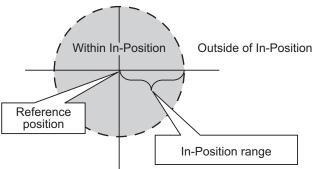
For the angle In-Position Judgment, if the  $\theta$  Command value is less than or equal to the ± In-Position range (sCALCVIRTUALMOVE\_PARAMS.InPosRange[1]) with respect to the reference mark position  $\theta$  value, it is within the In-Position. If it is larger than that range, it will be outside of the In-Position.
