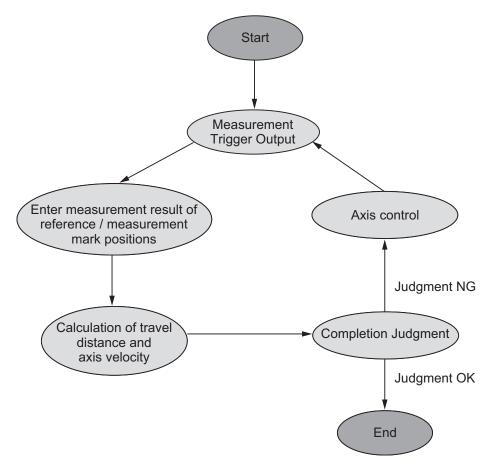
When it can be determined that the difference between the reference mark position and measurement mark position specified as the Completion Judgment target in sJUDGE\_PARAMS.TargetMark is all within the In-Position range (sJUDGE\_PARAMS.InPosRange), the alignment control is completed and alignment control in progress (Active) returns to FALSE.
