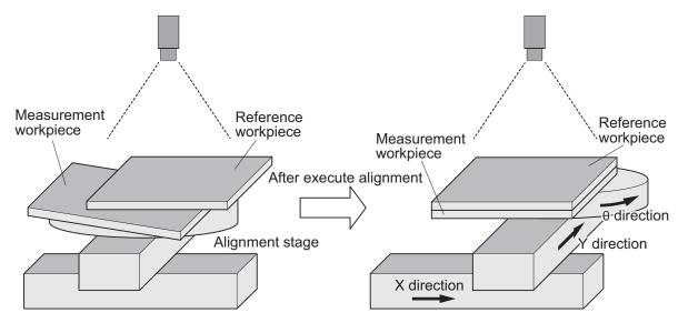
With this library, the stage is controlled using visual feedback of the measurement position/angle of the workpiece object as measured by the vision sensor.
