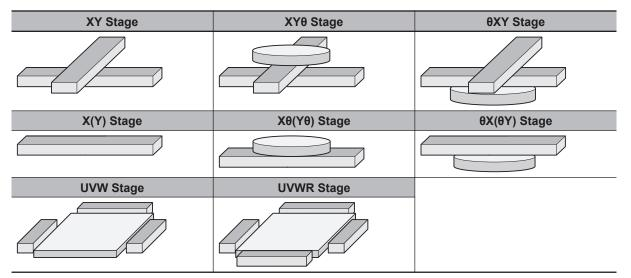
Regarding the control of  $\theta$  axis used in XY $\theta$ ,  $\theta$ XY, X $\theta$ (Y $\theta$ ),  $\theta$ X( $\theta$ Y) stage types, both direct drive (the drive system by which the  $\theta$  axis rotation is aligned to the rotary axis of a Servomotor) and Linear drive (the drive system by which rotation control of the  $\theta$  axis is done by linear movement) are supported.
