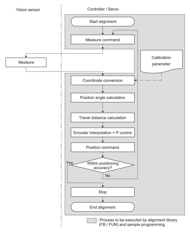
Alignment whereby measurement positions and reference positions for multiple points are aligned. The difference from 1 point is that the part to perform coordinate conversion and multipoint position angle calculation differs based on the measurement result of multiple points.
