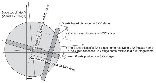
The X axis offset of a  $\theta$ XY stage home relative to a XY $\theta$  stage home
