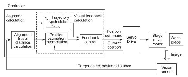
With the visual feedback control provided by this library, a trajectory of feedback control is generated for the calculated alignment travel distance. The generated feedback trajectory is given as a command to drive the stage with limits defined by the specified maximum acceleration/deceleration and maximum velocity.
