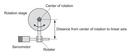
\*2. When setting the reference angle, if the  $\theta$  axis position of the reference angle does not match the home, please set that distance.
