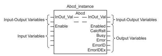
If an error occurs in the function block, the relevant error code and expansion error code are set in ErrorID (Error Code) and ErrorIDEx (Expansion Error Code). The error codes are retained even after Error changes to FALSE, but ErrorID is set to 16#0000 and ErrorIDEx is set to 16#0000 0000 when Execute changes to TRUE. 3
