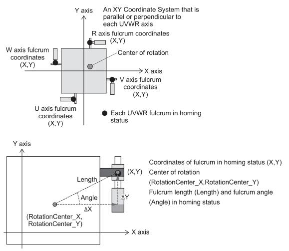
$\Delta X = X - RotationCenter_X$   $\Delta Y = Y - RotationCenter_Y$ Angle = tan<sup>-1</sup>  $\left(\frac{\Delta Y}{\Delta X}\right)$ Length =  $\sqrt{\Delta X^2 + \Delta Y^2}$
