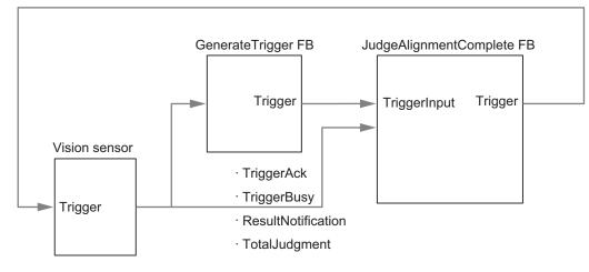
In-Position Judgment performed for the measurement mark position with respect to the reference mark position. This is the means for judging completion of alignment control.
