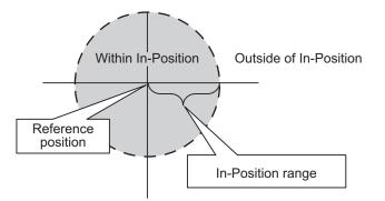
For the Angle In-Position Judgment, if the measurement mark position  $\theta$  value is less than or equal to the ± In-Position range (sJUDGE\_PARAMS.InPosRange[1]) with respect to the reference mark  $\theta$  position  $\theta$  value, it is within the In-Position. If it is larger than that range, it will be outside of the In-Position.
