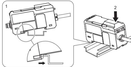
•How to install the amplifier slave unit
